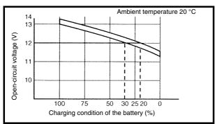
b. Check the charge of the battery, as shown in the charts and the following example.
