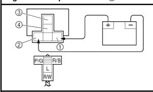
Does the radiator fan motor relay have continuity between red/white and blue?
