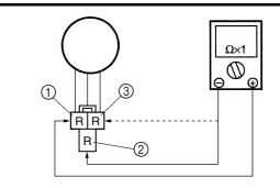
Measure the stator coil resistances.
