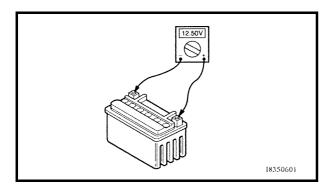
a. Connect a pocket tester to the battery terminals.
