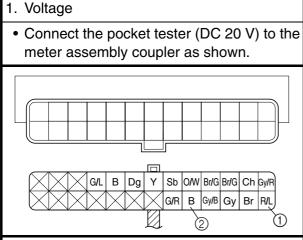
Positive tester probe  $\rightarrow$  red/blue ① Negative tester probe  $\rightarrow$  black ②
