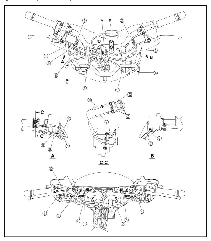
D After connecting the throttle cables, check the operation of the throttle grip and make sure that it returns to its home position easily after being released.
